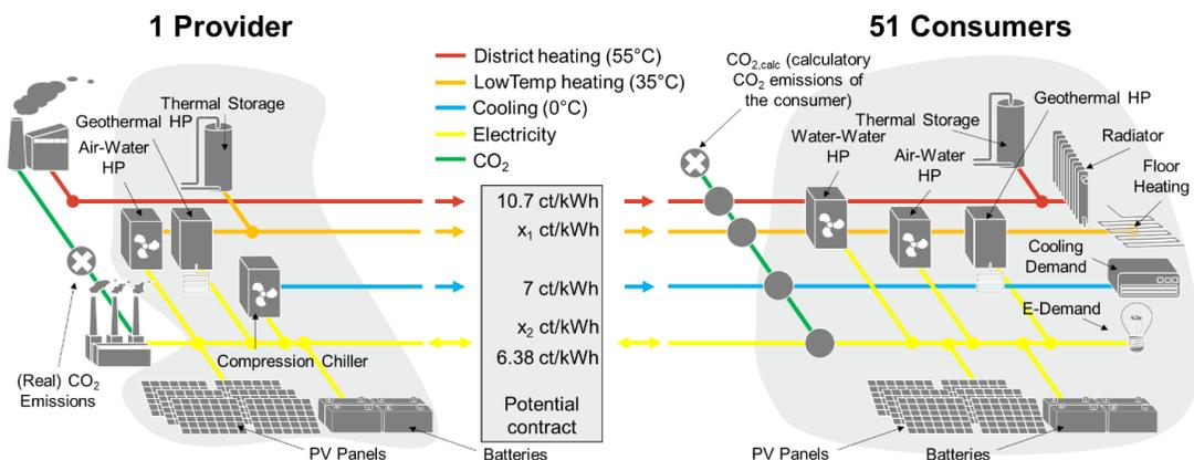
Figure 1. Decomposition of the optimization model into a provider and 51 consumer models interacting by a fixed contract.
